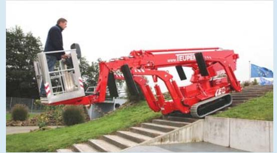
On the powerful track drive the LEO25Tplus can be maneuvered precisely. It even allows the machine climb steep slopes and stairs.
