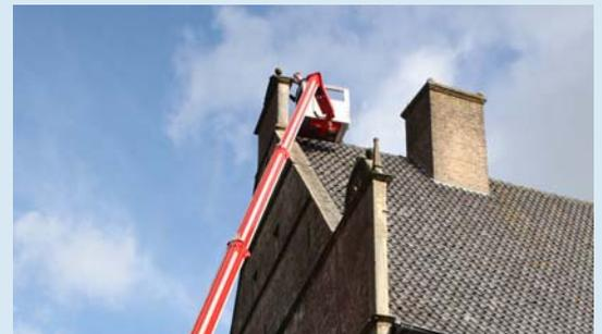
The LEO25Tplus features a 180° rotatable basket for more versatility when positioning the basket into tight spots, working alongside façades or in trees.
