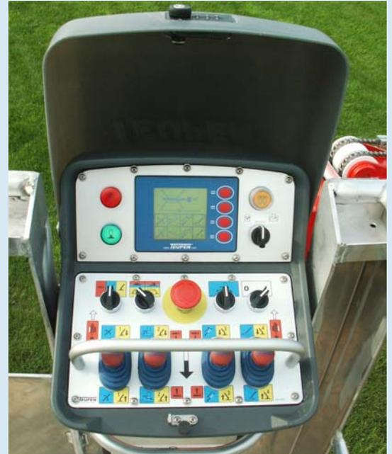
An interactive display in the control panel shows all available boom functions, safety information and allows error analysis.
